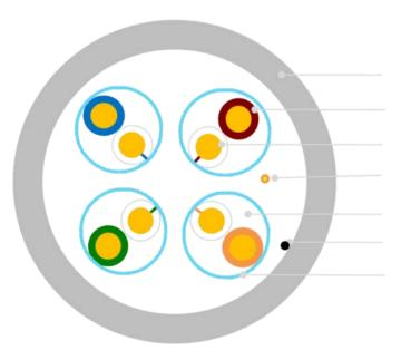
Jacket Insulation Conductor Drainwire Twisted Pair Ripcord Aluminum Foil Sheet
