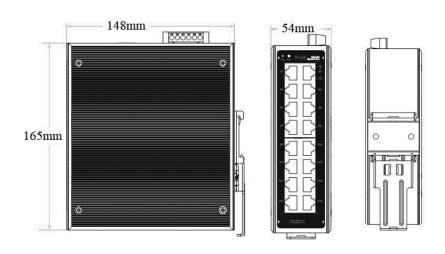
Dimensions Width: 54 mm Height: 165 mm Depth: 148 mm
